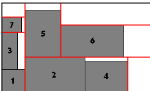
Figure 3: A sample packing produced by a Guillotine algorithm. The red lines denote the split choices.
